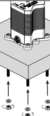
Secure valve to stringer by attaching washers and nuts to hardware stems. Tighten with wrench until snug.
