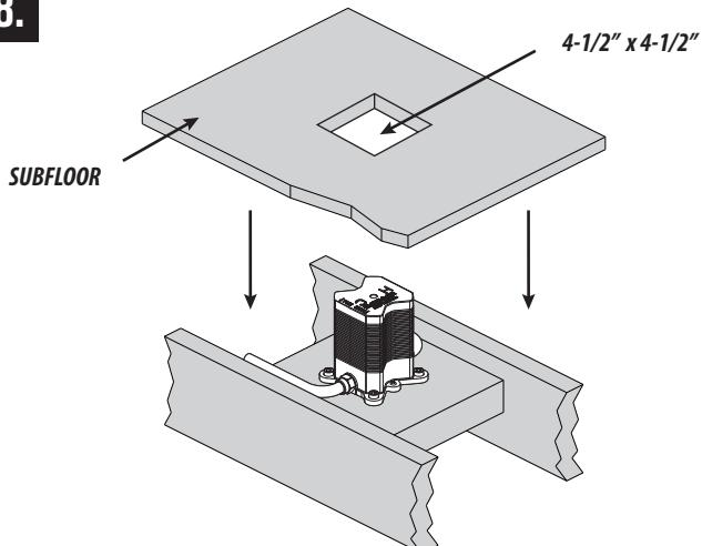
After leak test is complete, cut a square 4-1/2" x 4-1/2" hole into subfloor. Slide subfloor over plaster guard and secure.
