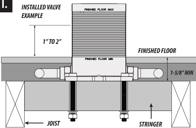
Before installation, determine the height of the valve position on stringer. For ease of trim installation, we recommend keeping the finished floor within 1" to 2" from the minimum valve height.
