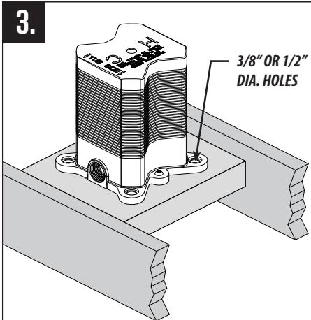
Mark valve hole positions with a pencil. Drill each of the four holes at 3/8" to 1/2" wide in diameter.
