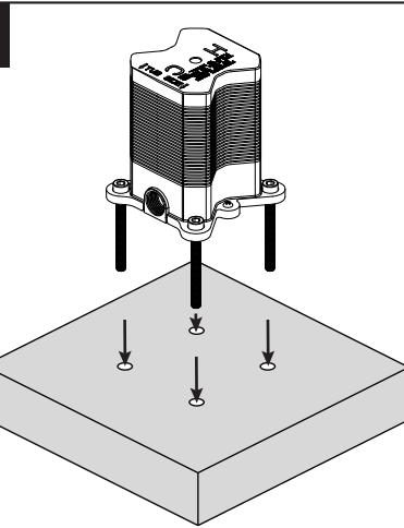
Slide valve and hardware through four holes. The cold inlet should be facing the tub.
