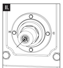
Reinstall temperature limit stop onto stem. Verify push override feature is free for movement.
