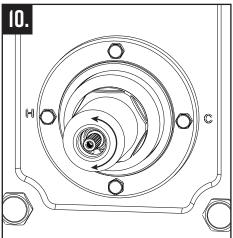
Rotate cartridge stem to adjust temperature: (clockwise = colder, counterclockwise = hotter).
