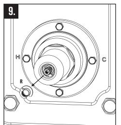
If temperature needs to be adjusted, locate temperature limit stop (R) in the end of the thermostatic hub. Remove from assembly. **NOTE**: The safe and factory set temperature is 100°F. Open shut-off valve and verify water temperature at outlet device by using a thermometer.
