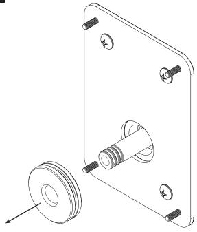
Pry the alignment spacer off of the injector and discard.
