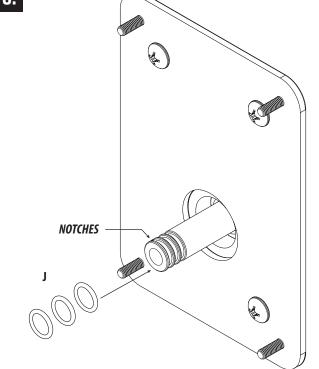
Use the provided 11.5mm I.D. X 2mm Wide O-rings (J). Install all three onto the injector and apply O-ring lube to them. Do not use petroleum based products on O-rings.
