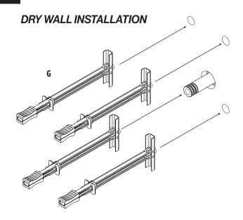
If there is no stud behind the back plate, utilize the provided high strength toggle anchors (G). Drill a 1/2" hole to push the toggle through. Once the toggle is through the wall, slide the cap down the straps until it is flush with the finish wall. Snap off the excess from the straps.
