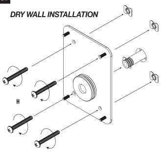
Using the provided 1/4-20 machine screws (H), secure the back plate flush to the finish wall using the toggle anchors. Ensure back plate is level.
