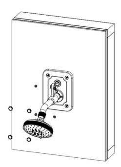
Using the provided nuts, tighten the trim onto the back plate. Once the trim is fastened to the wall use the provided deco nuts on all 4 corners. Thread them onto the threaded studs until they are flush with the trim plate.
