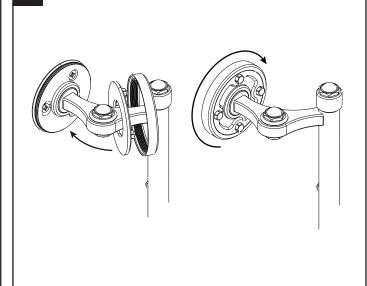
From the top dry bracket, carefully slide the ring and cover back over the deco nuts and screw onto base until snug.
