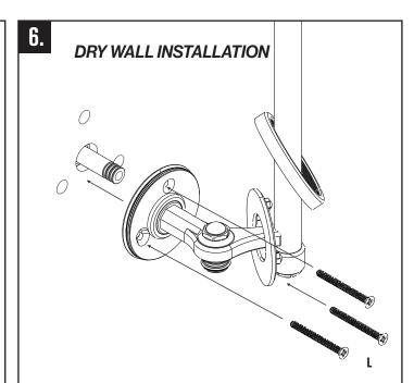
Apply non-petroleum based lubricant on the O-rings of the injector. Slide bottom bracket over the injector, ensure that it is level. Using the provided machine screws (L), secure both the dry and wet brackets to the finish wall using the toggle anchors.
