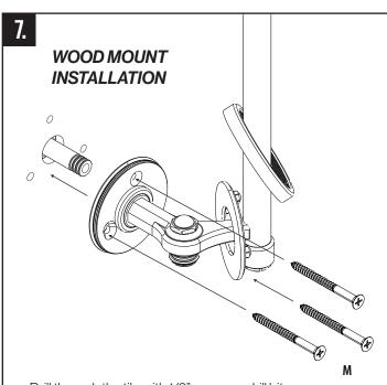
Drill through the tile with 1/8" masonry drill bit.
