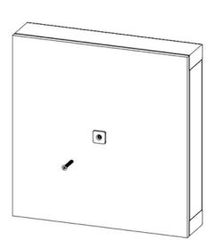
(DRYWALL): If there is no stud to mount to, drill a  $\frac{1}{2}$ " hole to push the supplied toggle through. Once the toggle is through the wall slide the cap down the straps until it is flush with the finish wall. Snap off the excess from the straps.
