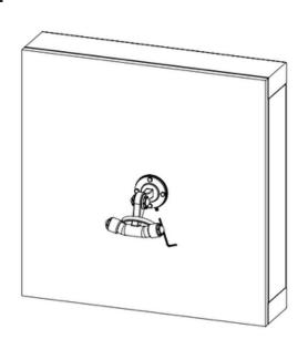
Place the robe hook onto the mount. Using the provided hex key, tighten the set screws down to secure the robe hook to the mounting tab.
