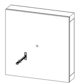
(STUD): Place the mounting tab with the groove facing down and the counter sink facing away from the wall. Use the supplied wood screw and fasten the tab to the wall.
