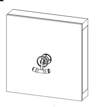
Carefully slide the escutcheon over the robe hook and thread onto the base.
