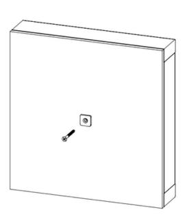
Using a 1/8" drill bit, predrill a hole on the center mark.
