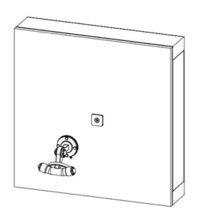
(DRYWALL): Using the provided  $\frac{1}{4}$ -20 machined screw, secure the mounting tab to the finish wall with the groove facing down.
